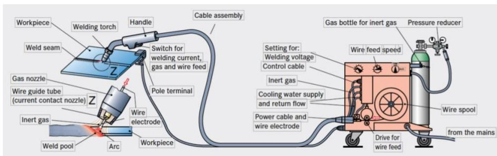
Graphic: Inert gas metal arc welding (TIG/TAG)
