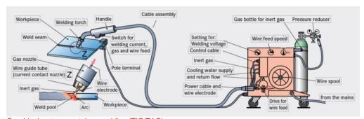
Graphic: Inert gas metal arc welding (TIG/TAG)
