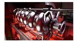
**BU:** Internally welded particle accelerator (cavity) in basic physics research
