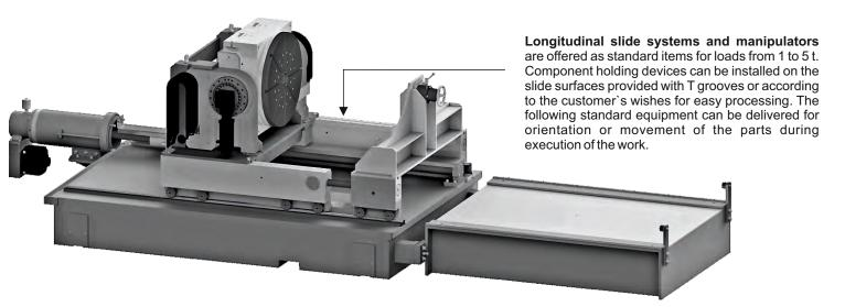
Compact slides with bridge and tailstock
