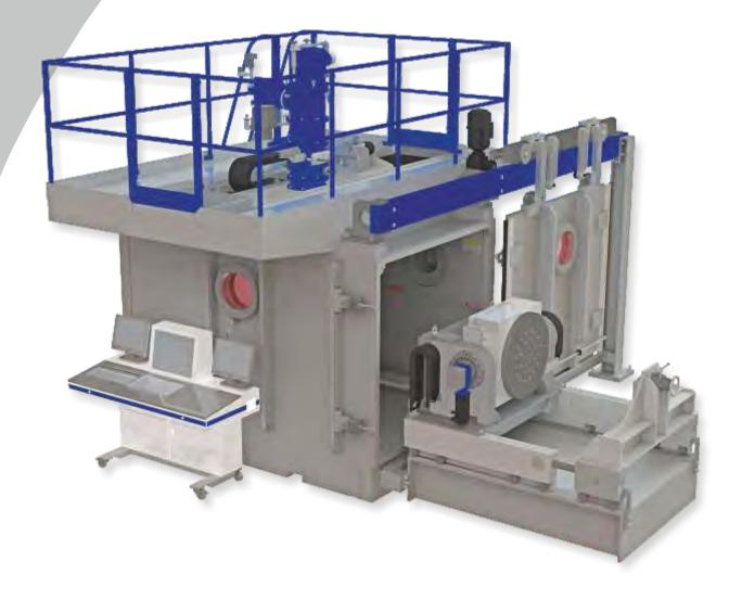
Chamber machines with longitudinal slide and 150 kV EB generator on a generator slide
