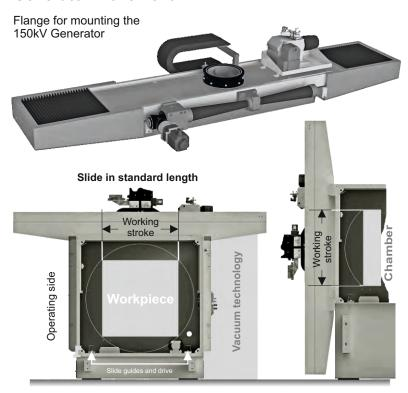
The generator chassis is an ultra-precise, vacuum sealing linear slide system with a travelling distance in the standard model which allows the EB generator to move over the entire width of the components so that transverse movements of the work pieces are avoided. Evacuation time and energy costs are reduced considerably by this reduction in the width and volume of the chamber and the productivity of the machine increases.
