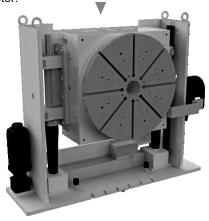
This rotating device can be mounted on a **hoisting slide** via ball screws with a precise drive on both sides as an option (as shown in the adjacent picture) - or with a **swivel unit with servo drive** for tilting the face plate by 90° (as shown) below.
