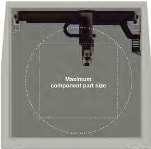
Design A: Longitudinal bridge travelling gear with a cross travelling gear and generator including a built-in rotating and swivelling axis on a telescopic vertical travelling gear
