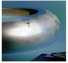
Combustion chamber housing 3,746 drill-holes with 0.9 mm diameter
