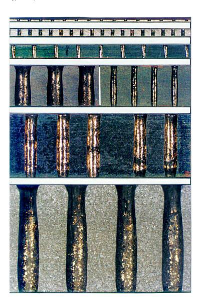
Cross-sections of EB drill-holes in CrNi steel
