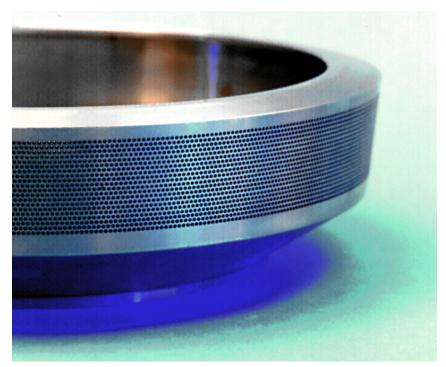
Spinner used in glass fibre production 25,600 drill-holes with 0.55 mm diameter
