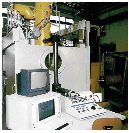
Control console of an EB drilling machine
