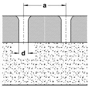
Limits for the distance between drill-holes
